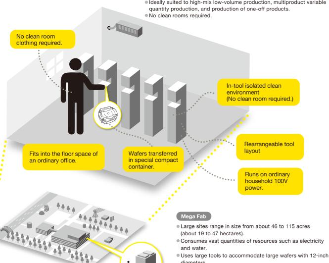
Minimal fab uses wafers with a half-inch diameter. These are very small compared to the 12-inch wafers used in mega fab facilities. Minimal fab's use of such small wafers makes it
